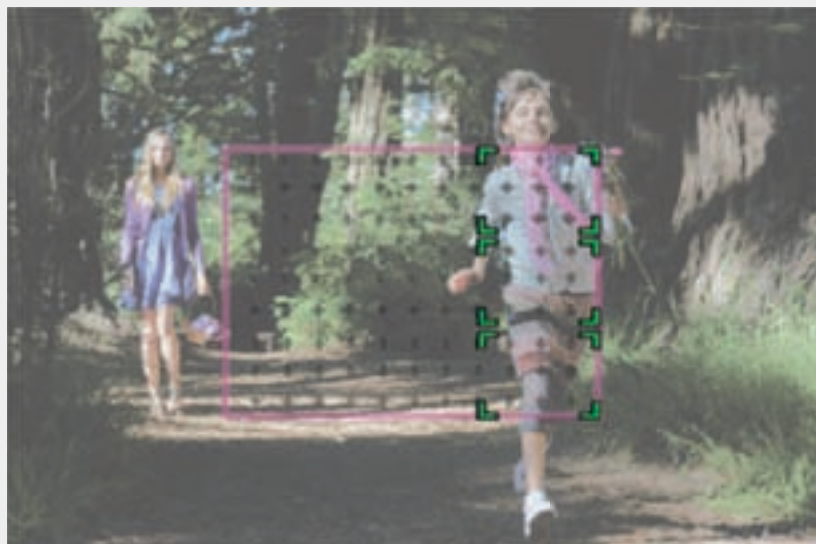
□ Area covered by 99-point phase-detection AF.
