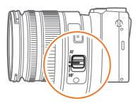
When your lens has no AF/MF switch, select an AF mode from the camera menu.
