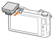
3 Lock the flash into place by turning the hot-shoe fastening dial clockwise.
