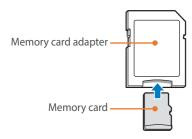
To read data with a computer or memory card reader, insert the memory card into a memory card adapter.
