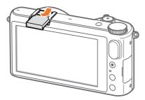
Mount the flash by sliding it into the hot-shoe.
