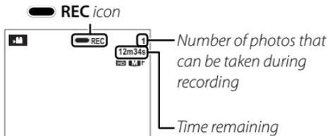
To end recording, press the
