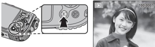
Press the selector right to view pictures in the order recorded, left to view pictures in reverse order. Keep the selector pressed to scroll rapidly to the desired frame.
