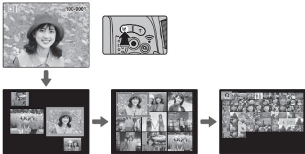
When two or more images are displayed, use the selector to highlight images and press **MENU/OK** to view the highlighted image full frame. In the nine- and hundred-frame displays, use the selector to view more pictures.
