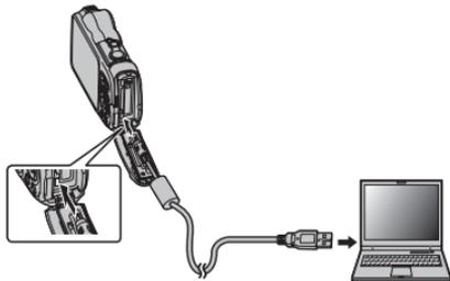
Ⓢ Be sure the battery-chamber cover is open before attempting to open or close the connector cover.
