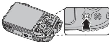
Press the **▶** button again or press the **ON/OFF** button to turn the camera off.
