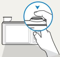
Half-press **[Shutter]** and adjust the focus. The camera adjusts the focus and exposure automatically.
