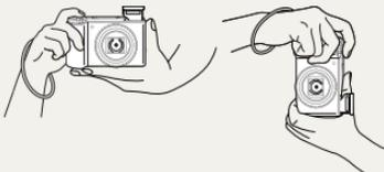
Ensure nothing is blocking the lens, flash, or microphone.
