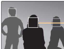
The face nearest the camera or nearest the center of the scene appears in a white focus frame and the rest of the faces appear in gray focus frames.
