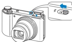
When the flash unit is closed, the flash does not fire regardless of the selected option. When the flash unit pops up, the flash fires according to the selected option.
